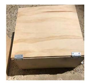
16. Remove excess screw nubs protruding into the inside of the box with a Dremmel tool fitted with a metal cutting bit. Fill holes with wood putty and sand.
